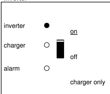
The inverter is switched on and supplies power to the load. Battery operation.
