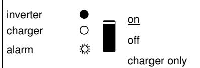
The inverter is switched on and supplies power to the load.
